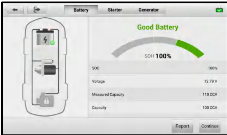
Figure 13-7 Battery Test Results Screen
