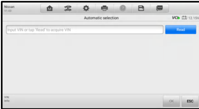
Figure 6-8 Automatic Selection in TPMS Application
