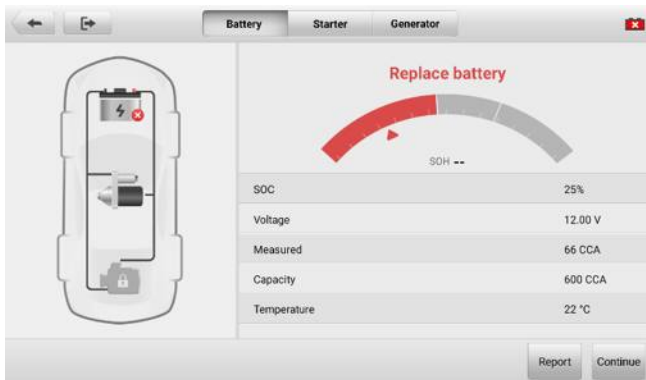
Figure 8-7 Battery Result Screen
