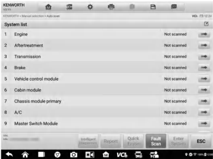
Figure 5-4 Sample Fault Scan on System List Screen 1
