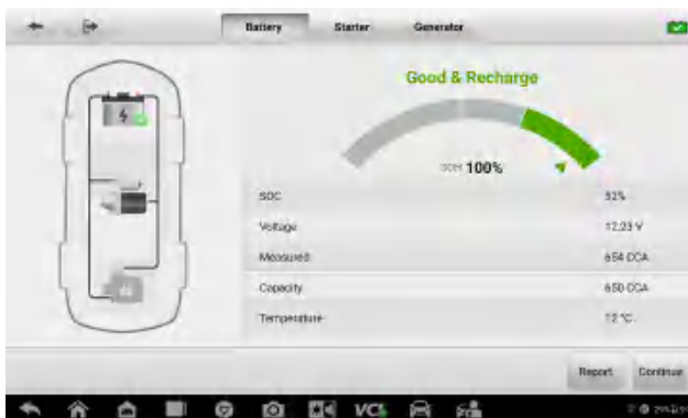
Figure 6-7 Battery Test Results Screen
