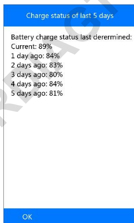
Figure 5-52 Sample Battery Charge Status of Last 5 Days
