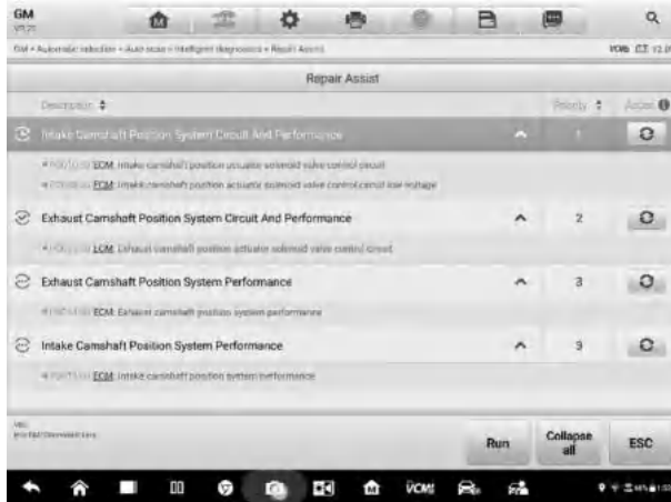
Figure 5-21 Sample Repair Assist Screen 2
