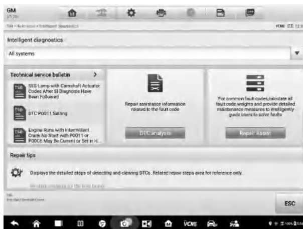
Figure 5-20 Sample Repair Assist Screen 1
