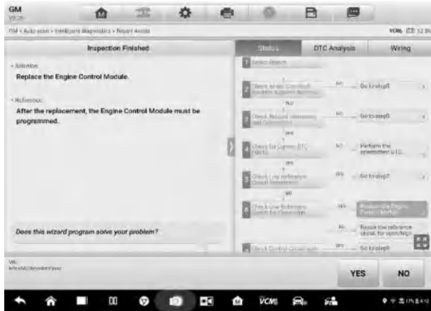
Figure 5-28 Sample Repair Assist Screen 9
