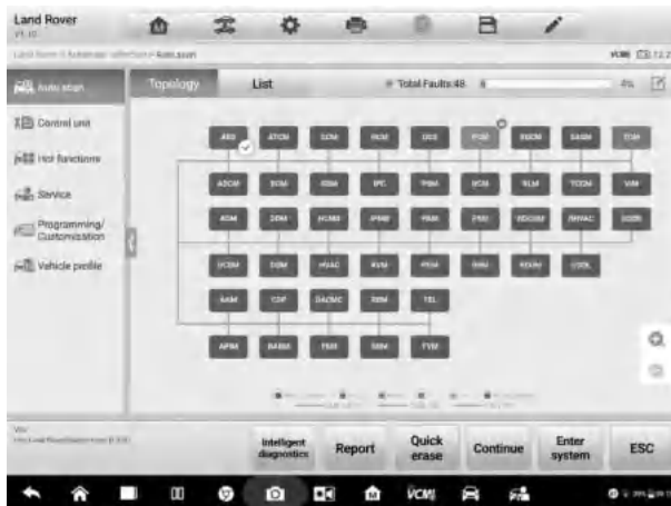
Figure 5-6 Sample Fault Scan on Topology Screen
