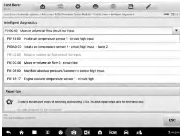
Figure 5-16 Sample Vehicle System and Detected DTC(s) Screen
