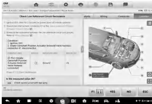
Figure 5-24 Sample Repair Assist Screen 5
