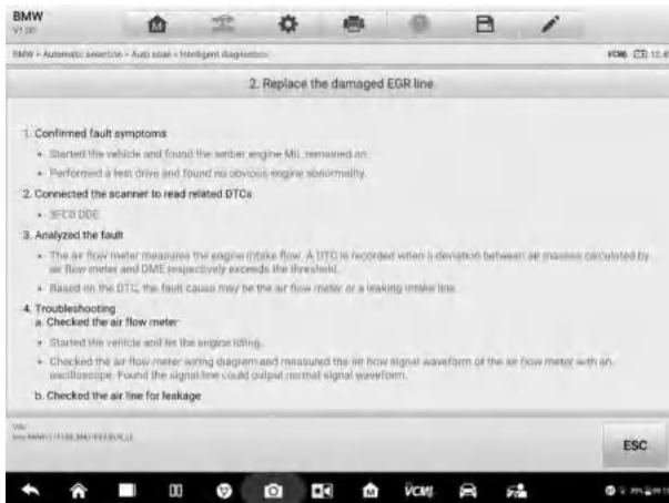
Figure 5-30 Sample Repair Tips Description 11 (Text)
