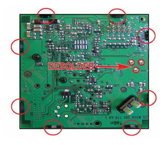
Please remove the regulator marked **X** and discard. Once removed reassemble the PCB taking care of the switch marked in the **Red Circle**, making sure it is not damaged.
