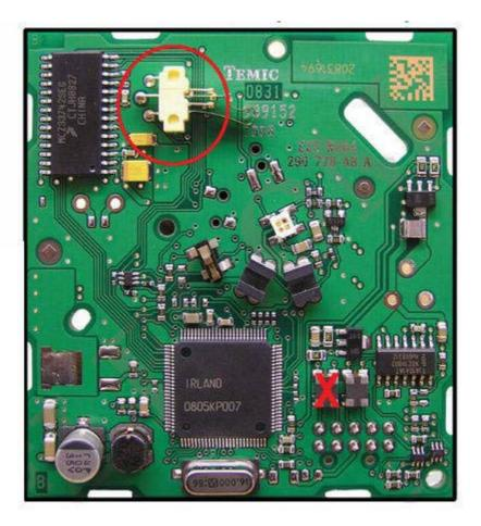
Connect wires from Can Filter to EZS as shown below. Please make sure that the top two left resistors shown **X** below are not present on the Can Filter, if so please remove and discard. Once all wires are connected try in car before completing. It is advisable to insulate the Can Filter with heat shrink insulation tape. Finally fix the Can Filter to the EZS's PCB with doubled sided tape
