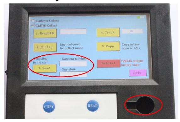
4, After crack Original key , put the original key hole
