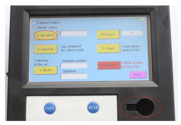
3.2 • Put the new key vertically into the bottom right corner of the hole, click on "Conf ig". Note: Do not going to be flat on the hole nearby, this is not easy to read information inside the chip.
