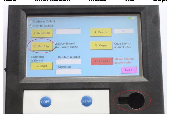
3.3 Use new car key collect information in car, first of all, take a key blank, put the new key into the key blank, insert the car key hole, four consecutive starts, each time interval of 3-5 seconds
