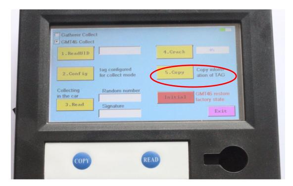
6、 If in the process, chip key copy failed, put the key into bottom right corner of the hole, click on "Initialize", restart again from the first step.
